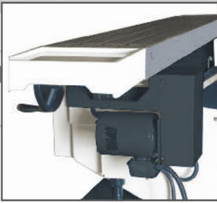
X & Y axis automatic feeds driven by 1/2HP motor and inverter
