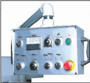
Control panel with speeds tachometer
